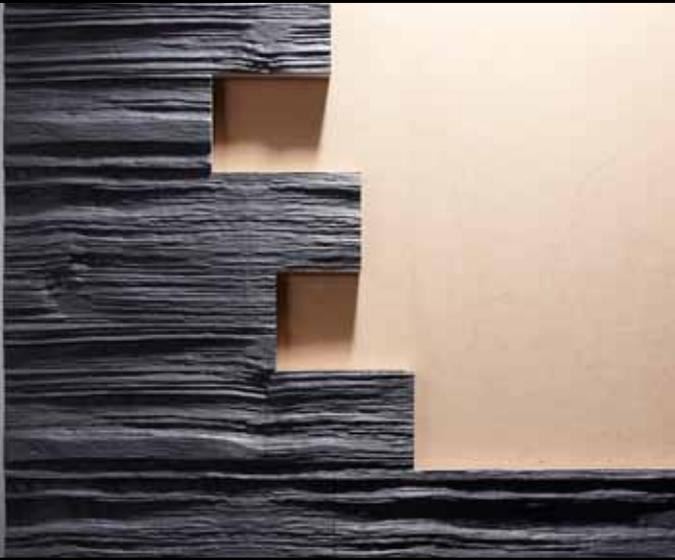
By shortening, sliding and turning the individual segments, you can create a uniform fiddleback pattern with an emphasis solely on the vertical graining.
