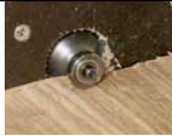
Refinish the excess length with a profile cutter. Primarily use small tool profiles. A ball bearing guide ensures a smooth tool guidance.
