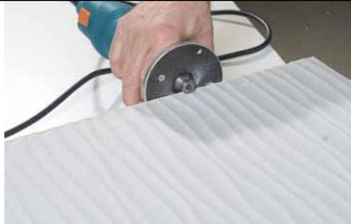
To avoid damages of the surface chamfer against your tools rolling direction.
