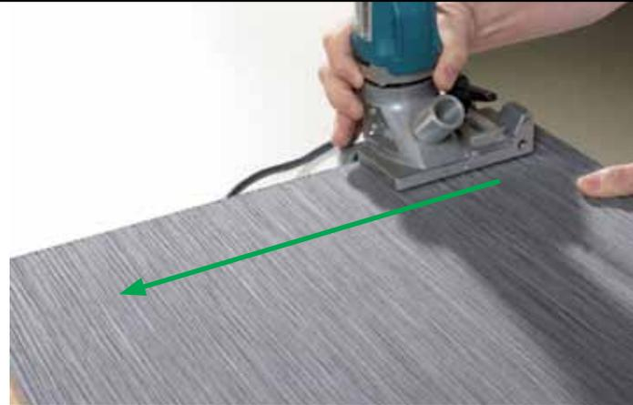
Primarily use small tool profiles for bevels or radius such as millers for 45° bevels or for 1.5 to 3mm radius.
