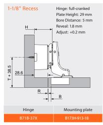
NOTE: B = Bore Distance | H = Plate Height | R = Reveal | T = Door Thickness
